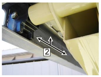
Figure 6-3. Upper Slide Pad Channel
