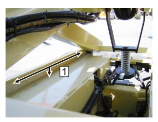
Figure 6-2. Lower Slide Pad Channel
