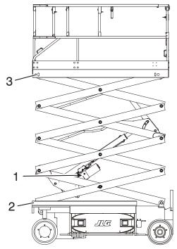
Figure 6-1. Lubrication Diagram
