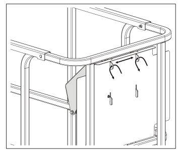
Figure 4-2. Securing Control Station to Platform
