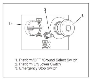
**Figure 3-1. Ground Control Station**
