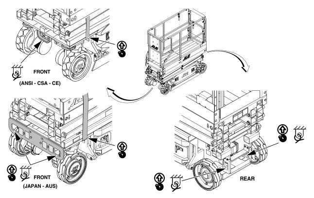
Figure 4-3. Lifting and Tie Down Diagram
